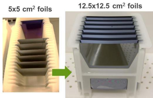
**Figure 3.** Change in foil size from 25 to 156.25 cm<sup>2</sup>
