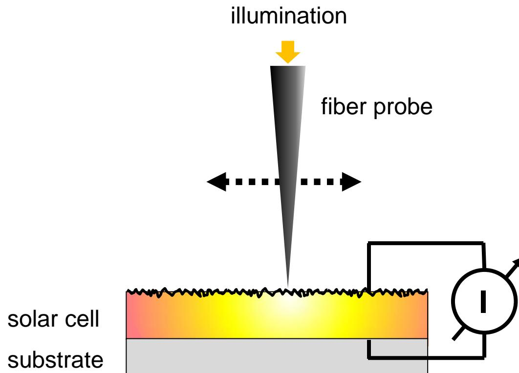
Use the sample (solar cell) as detector
