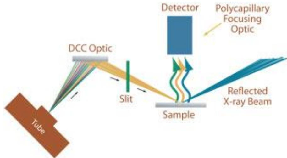
An incident beam impinges upon a sample at angles below the critical angle of external total reflection for X-rays resulting in **reflection of almost 100% of the excitation beam photons.**
